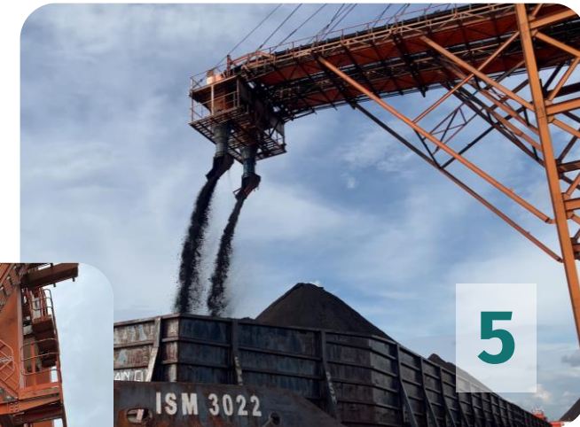
Kramasan Port with 3 lines barge loading conveyors
